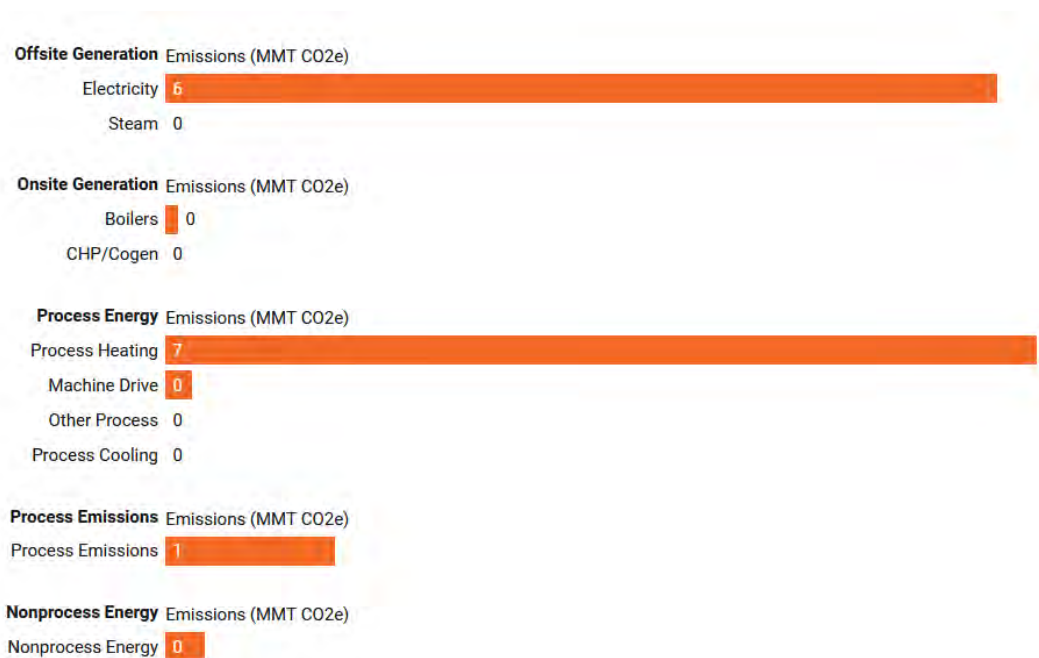
Figure 22: Glass sector sources of GHG emissions in 2018, by major end use. Source: U.S. DOE, Manufacturing Energy and Carbon Footprint: Glass Sector.
